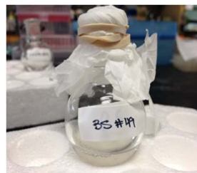
Round-bottom flask (lyophilizer bulb) with aqueous fraction prior to lyophilization. Steps 16 and 18.
